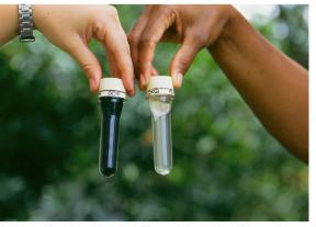
Simple presence/absence vials are being used by the Fijian communities of Vanisinu and Nalase to test their drinking water quality. This simple hydrogen sulphide strip test is assed to help households test their own water supplies. Mier comminated with faced coliform unres black within a couple of days.
