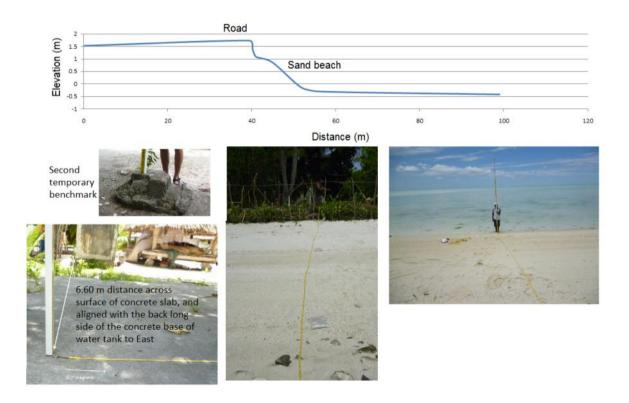
Figure 7. Profile of transect surveyed across the road margin at Tabon-ke-bike (Site 1b).
