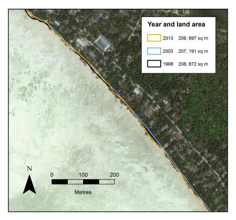
**Figure 13**. GIS analysis of shoreline change 1998-2013 at Nooto Ramsar site southern lagoon shore beach, of the southern red box area shown in Figure 12. The background image is 2013, and the land area calculations are based on the land area shown in the image.
