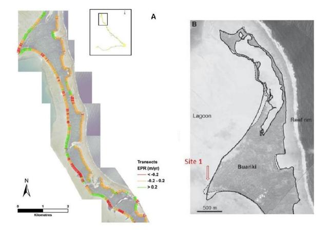
**Figure 3.** Shoreline changes at Buariki. A) From 1968-1998, adapted from Figure 5 of Biribo and Woodroffe (2013). B) From 1969-2004, adapted from Figure 6b of Webb and Kench (2010), with Site 1 of this report identified in red.
