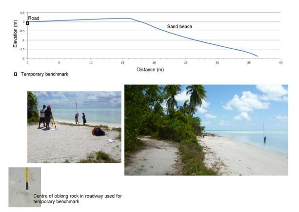
Figure 5. Profile of transect surveyed at Tabon-te-bike site 1a.
