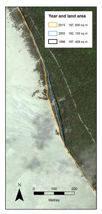
**Figure 14**. GIS analysis of beach shoreline change 1998-2013 at Nooto Ramsar site northern lagoon shore beach, of the northern black box area shown in Figure 12. The background image is 2013, and the land area calculations are based on the land area shown in the image.
