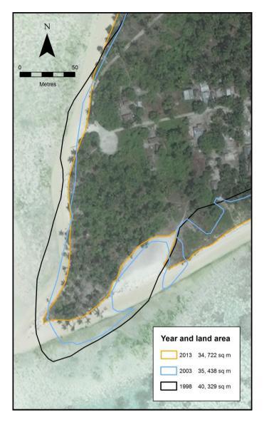
**Figure 4**. GIS analysis of shoreline change 1998-2013, Tabon-ke-bike, Buariki. The background image is 2013, and the land area calculations are based on the land area shown in the image.
