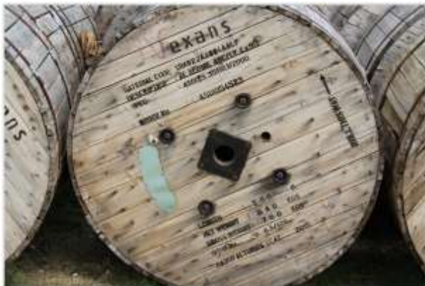
Photo 9: Project LV ABC Conductor
