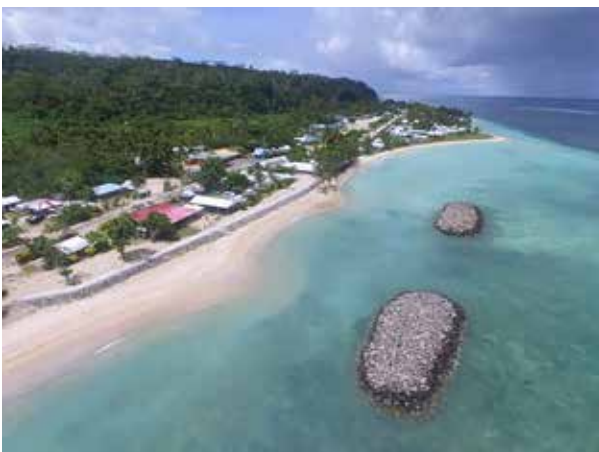
Figure 3-5 Salients Created in the Lee of Offshore Breakwaters at Manase Beach, Samoa
