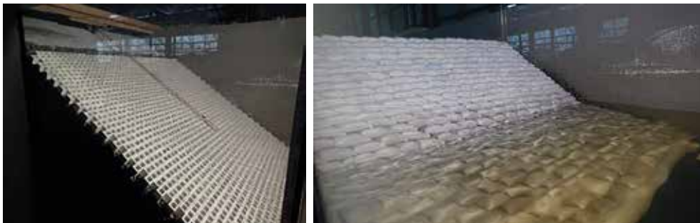
Figure 3-8 Model Concrete Masonry Block and Hand Placed Geotextile Container Revetment in Wave Flume
