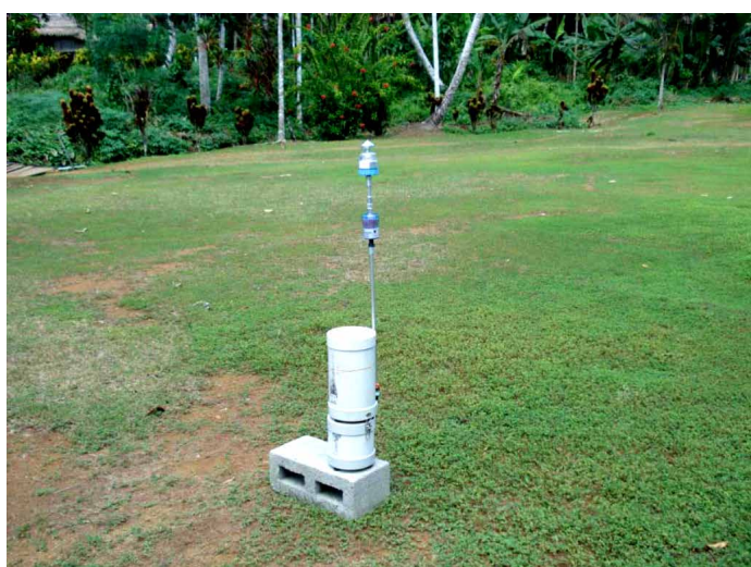
FIGURE 2.5. MicroVol Sampler use for PM10 monitoring at Leleghia, Santa Isabel (© SMM Solomons Ltd)
