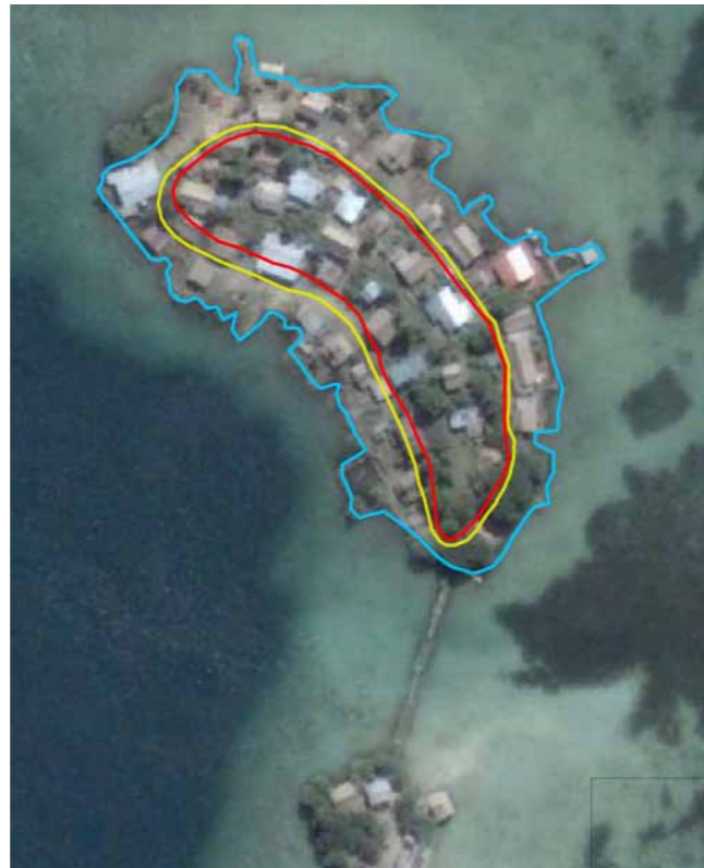
Topographic survey results from Nusa Hope showing high tide mark, 0.5 m and 1 m contours. Sea level is likely to rise by 0.5-1m over the next 100 years.
