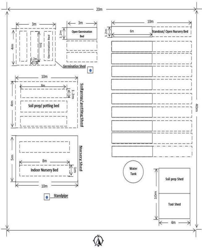
Figure 1: Layout of the BNHP Nursery (not drawn to scale). Note existing structures are in bold lines. Structures that require extension work are in dashed lines. The nursery shed requires new shed nets and beds. Soil preparation/potting shed and germination shed are new structures required by the BNHP nursery with indoor beds.
